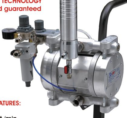
Recommended for joinery and light carpentry. It starts working at a pressure of 0.2 bar, feeding up to two spray guns.
